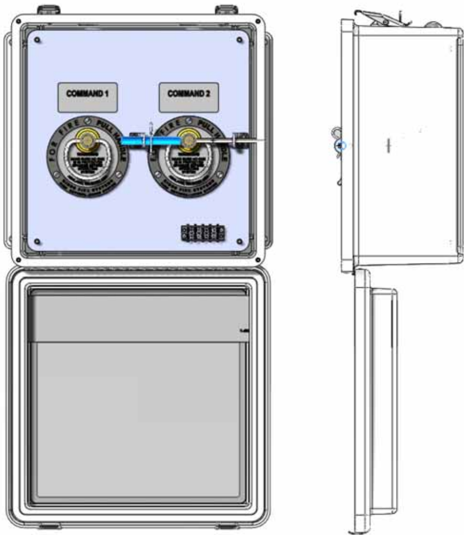
Figure 4-4. Fiberglass IMO Releasing Cabinet for Cable Release
